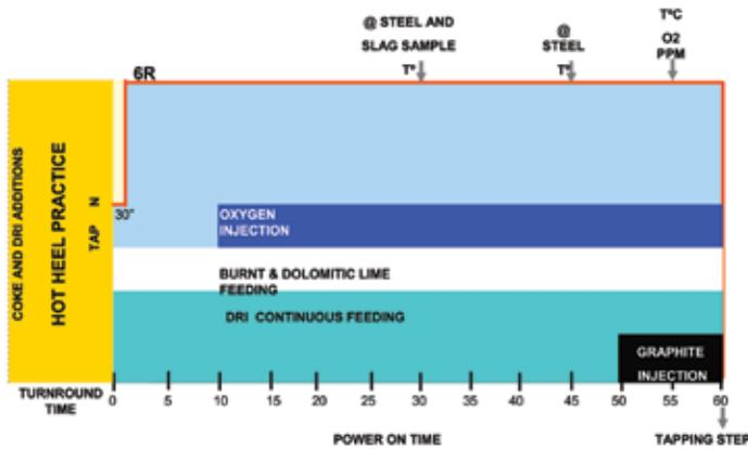
FIGURE 2 Melting pattern used for 100% DRI melting.
