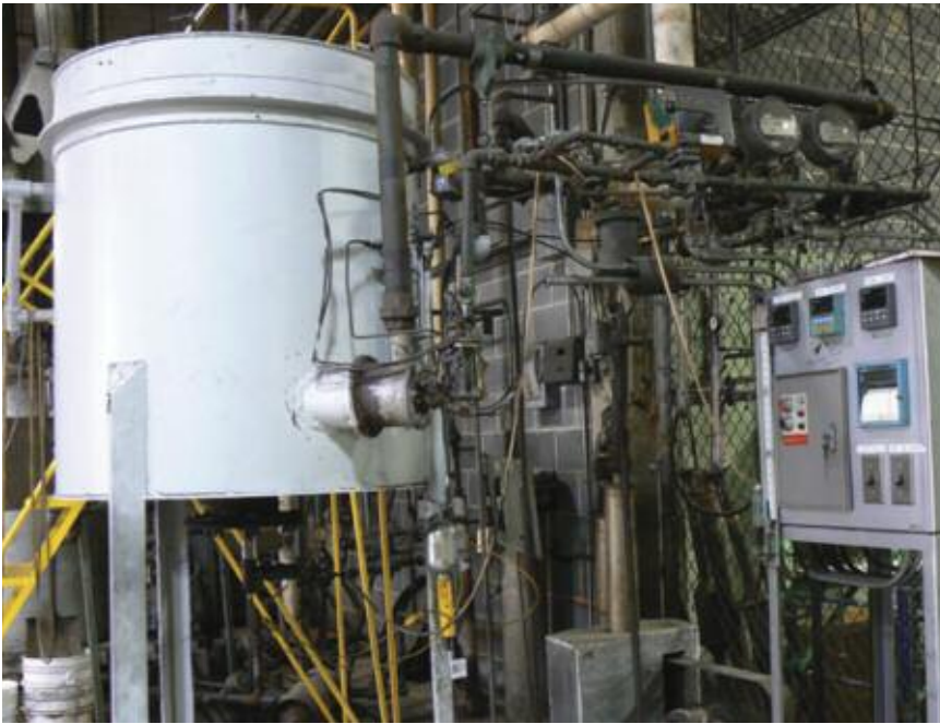
Figure 2 - Hot Load Test for Clustering and Reducibility
