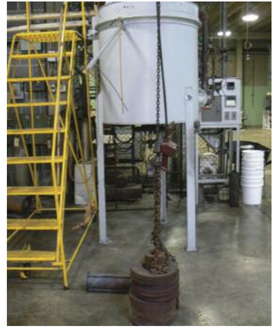
Figure 3 - Hot Load Test Showing Weights for Load
