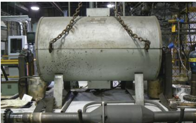
Figure 1 - Linder Test for Low Temperature Disintegration
