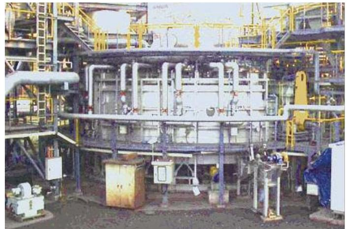
Figure 1 - Kakogawa Works FASTMET® Pilot Plant
