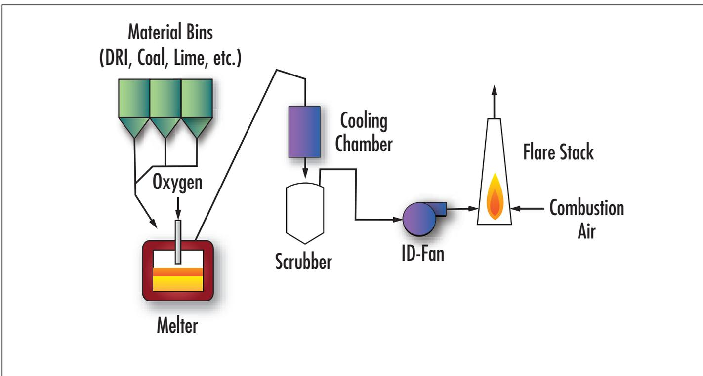
Figure 6 - Process Flowsheet of the Coal-based Melter
