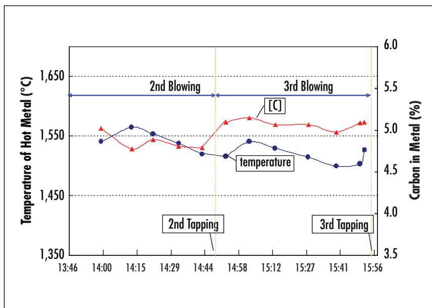
Figure 7 - Transition of Metal Temperature and Carbon Content
