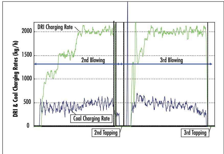
Figure 8 - Transition of DRI and Coal Charging Rates
