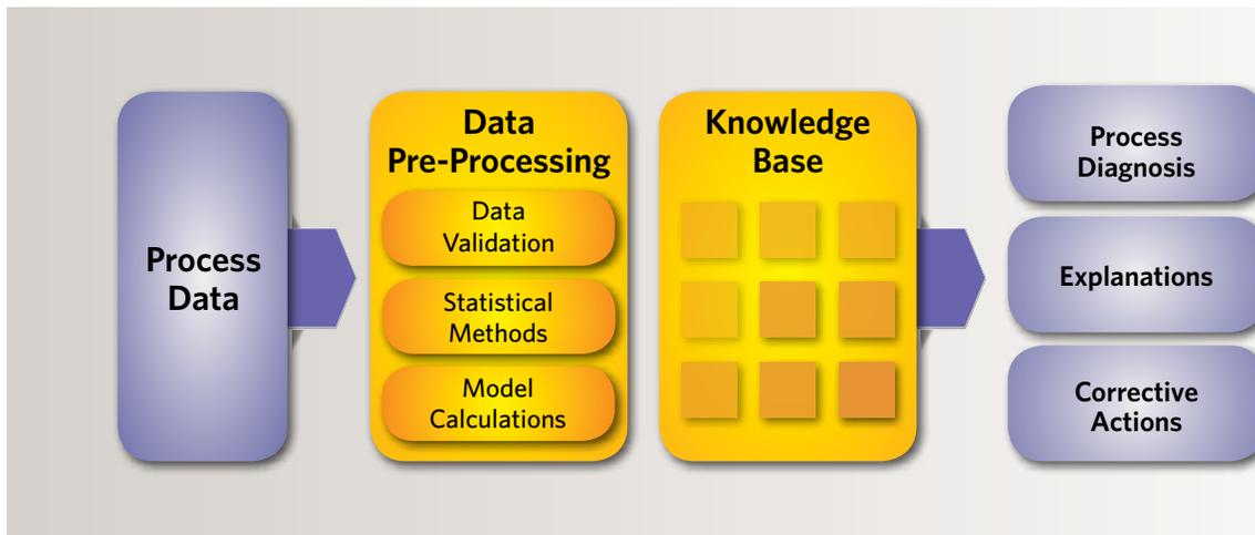
FIGURE 6 SIMPAX Expert System Structure
