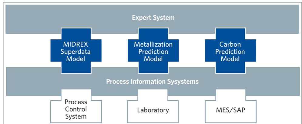
FIGURE 1 Next Generation SIMPAX Application Software Structure
