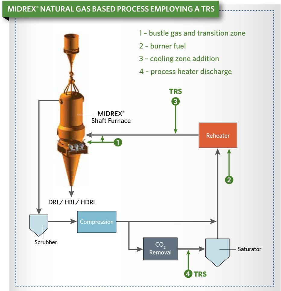
FIGURE 6 MIDREX® Natural Gas Based Process Employing a TRS
