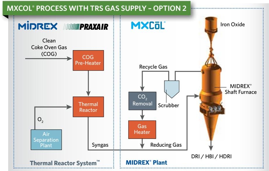
FIGURE 4 MXCOL® Process with TRS Gas Supply - Option 2
