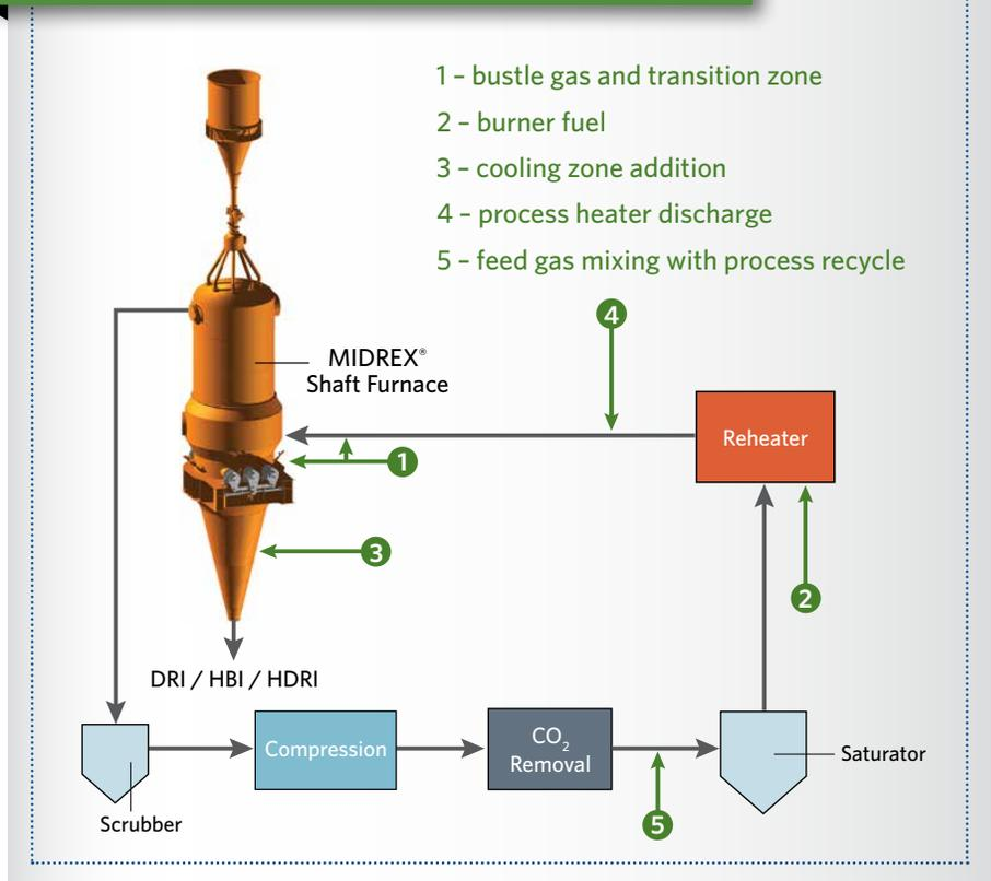
FIGURE 2 Potential Use Points in the MXCOL Process
