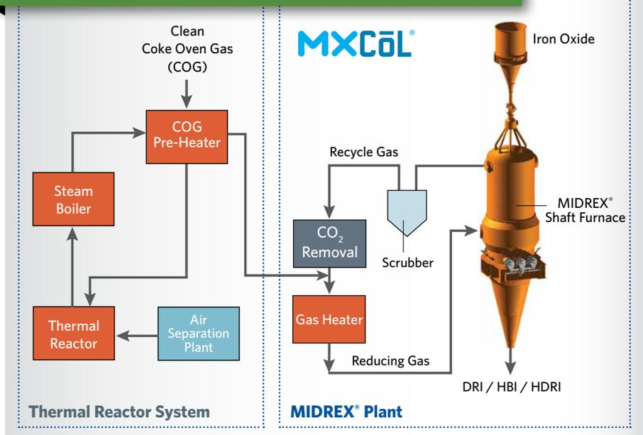
FIGURE 3 MXCOL® Process with TRS Gas Supply - Option 1
