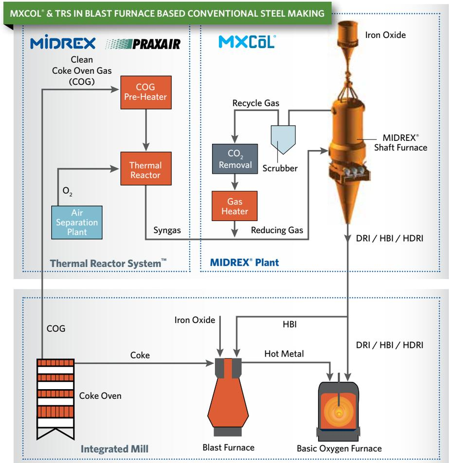
FIGURE 5 MXCOL® and TRS in Blast Furnace Based Conventional Steel Making
