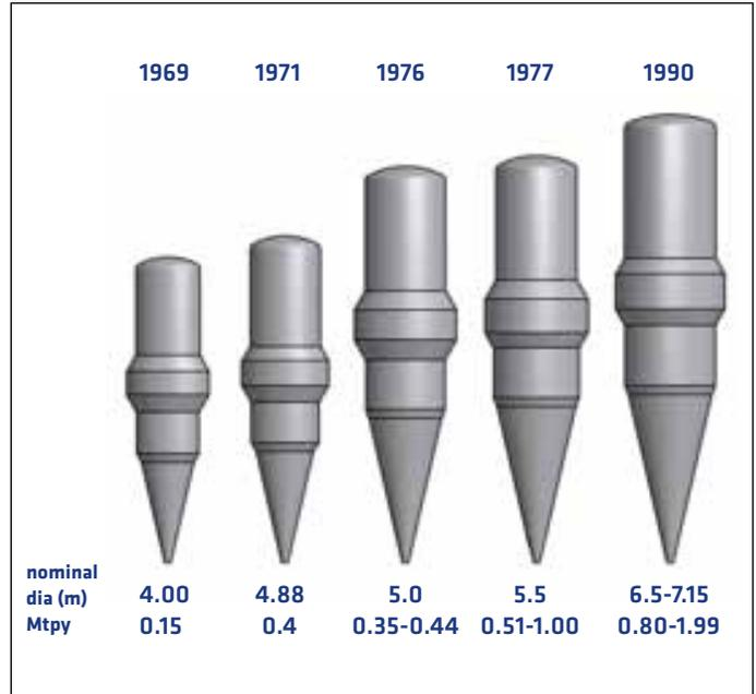
FIGURE 5 MIDREX Furnace Sizes (to scale) and Capacities
