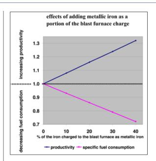
the major integrated steelmakers have conducted extensive tests (hundreds of thousands of tons of HBI each) with the focus being CO, savings. And, in China, where over half of the world's iron is made, a major feasibility study regarding CO2 saving by the steel industry targeted blast furnace usage of HBI.
