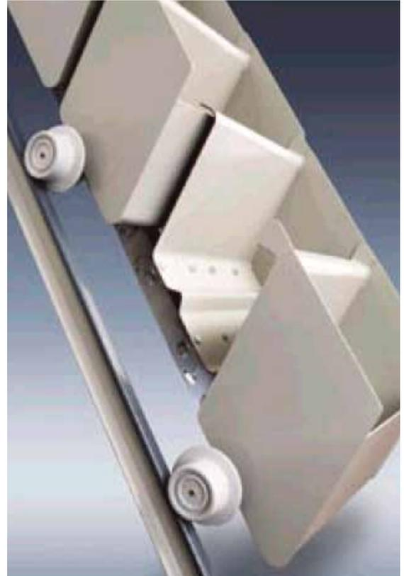
FIGURE 3 Aumund Bucket Conveyor System
