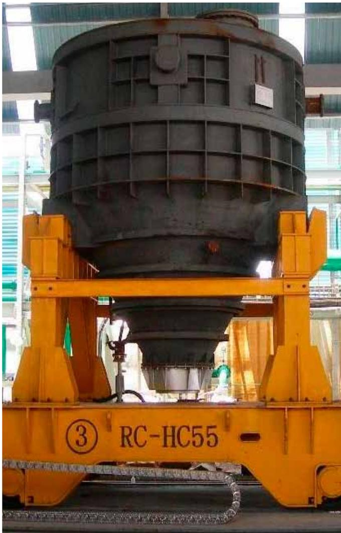
FIGURE 2 Hot Transport Vessel at LION
