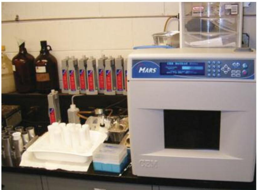
Figure 5 - Microwave Digestion for the ICP
