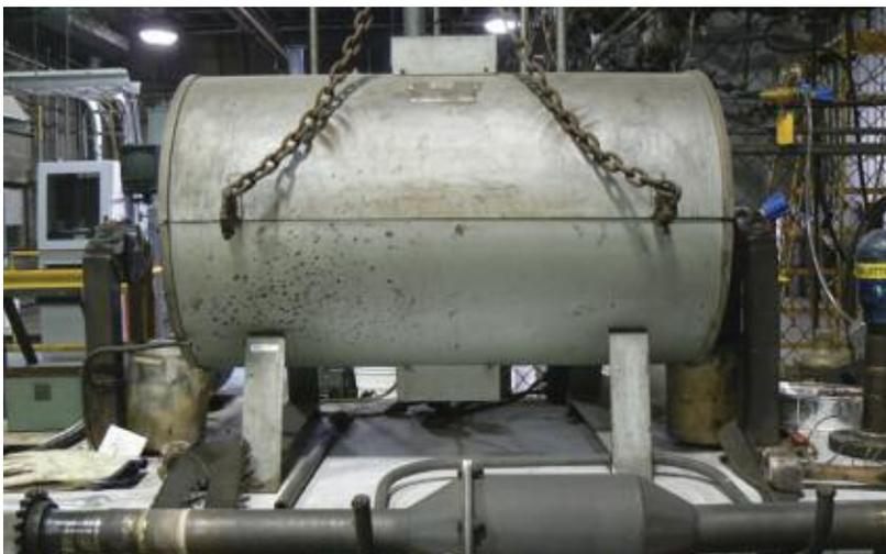
Figure 1 - Linder Test for Low Temperature Disintegration
