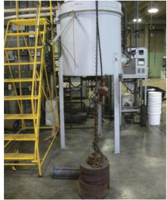
Figure 3 - Hot Load Test Showing Weights for Load
