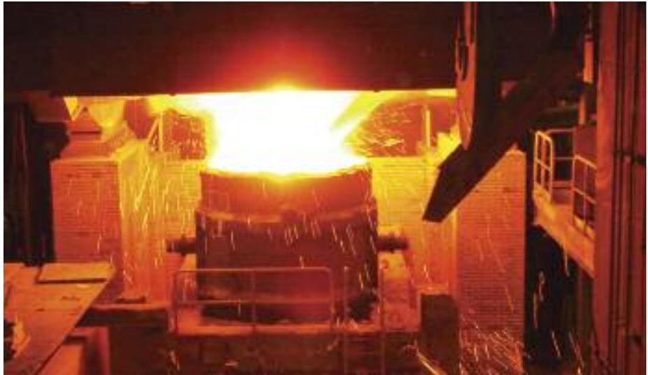
Figure 4 - Qatar Steel: Molten Steel Tapping at EAF2R
