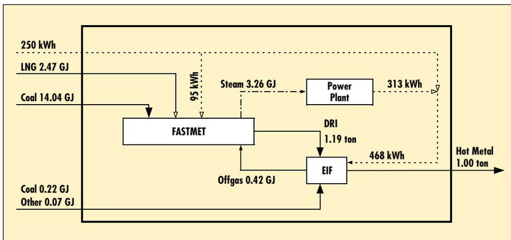
Figure 11 - Energy balance of FASTMELT® (500,000 t/y)
