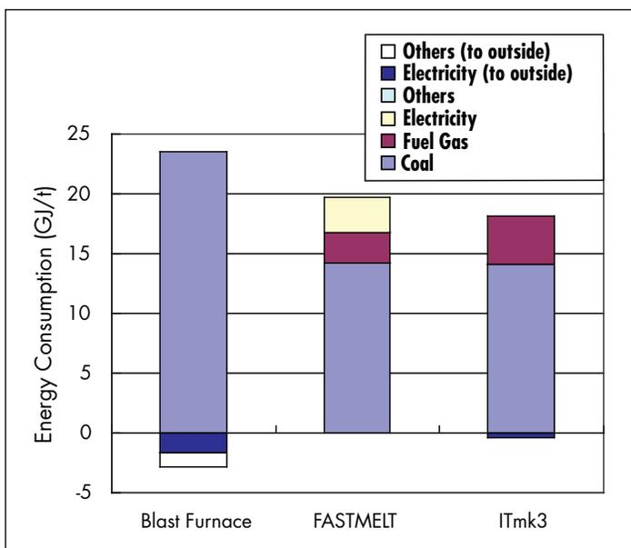
Figure 13 - Energy consumption of ironmaking processes
