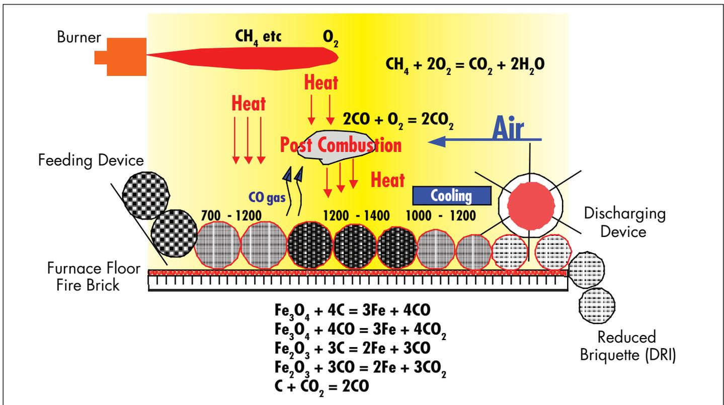
Figure 4 - Schematic drawing of reduction in RHF
