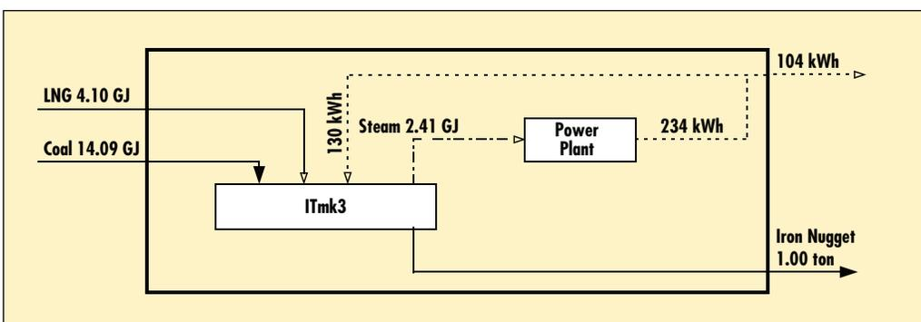
Figure 12 - Energy balance of ITmk3® (500,000 t/y)
