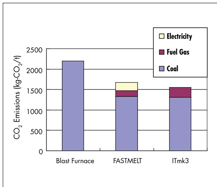
Figure 14 - CO<sub>2</sub> emissions of ironmaking processes
