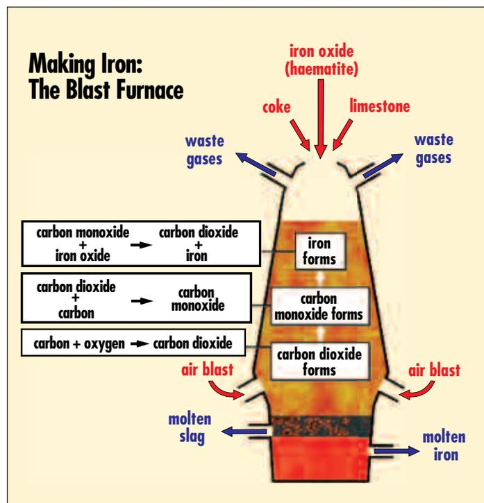
Figure 1 - Blast Furnace
