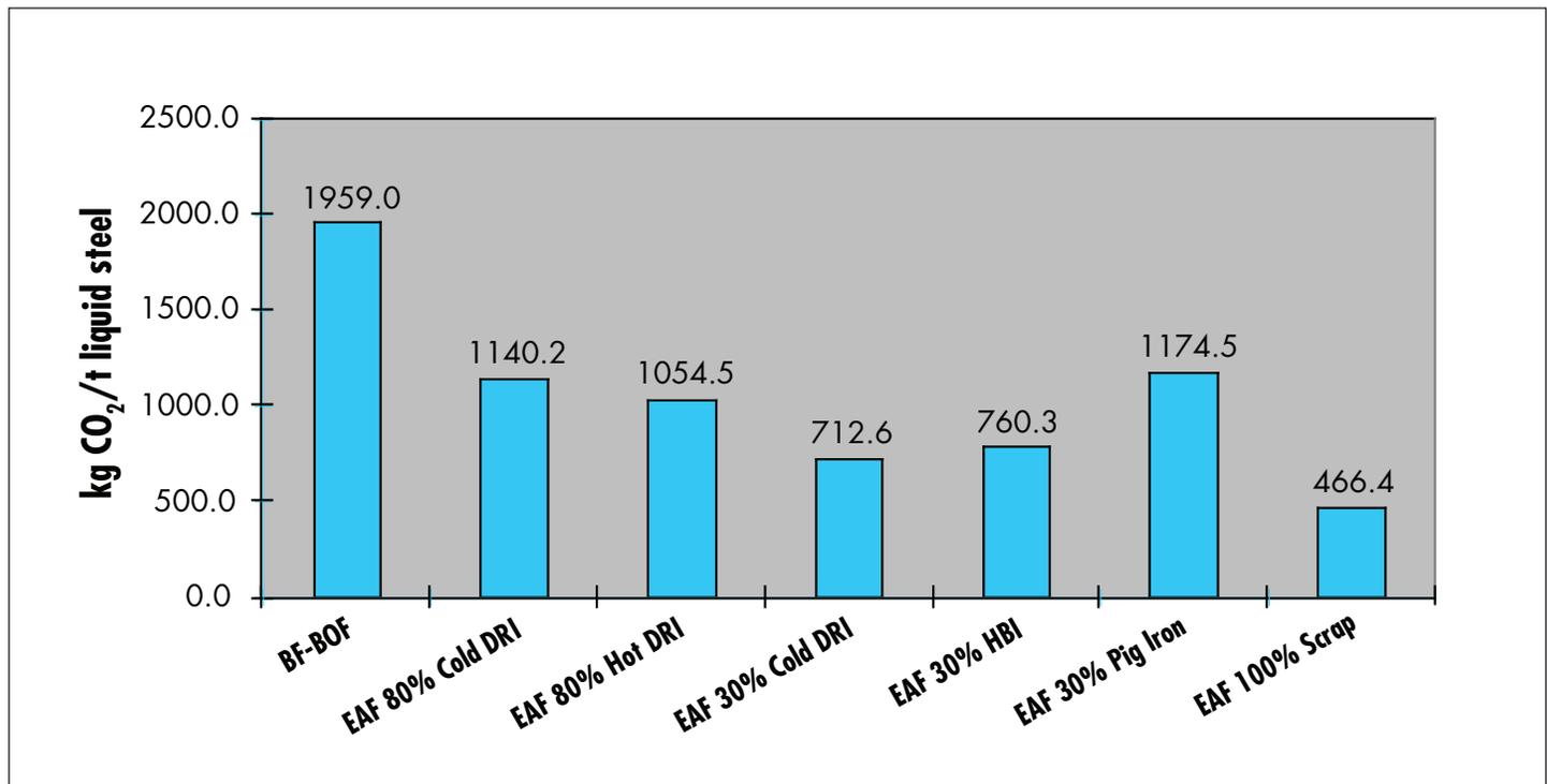
Figure 3 - Carbon Emissions for Steelmaking Routes
