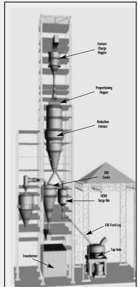
Typical HOTLINK arrangement with transformer located underneath the DR furnace
