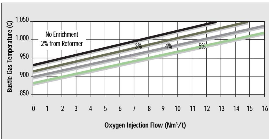
Figure 3 Temperature Rise with Oxygen at Various Bustle Gas Hydrocarbon Levels
