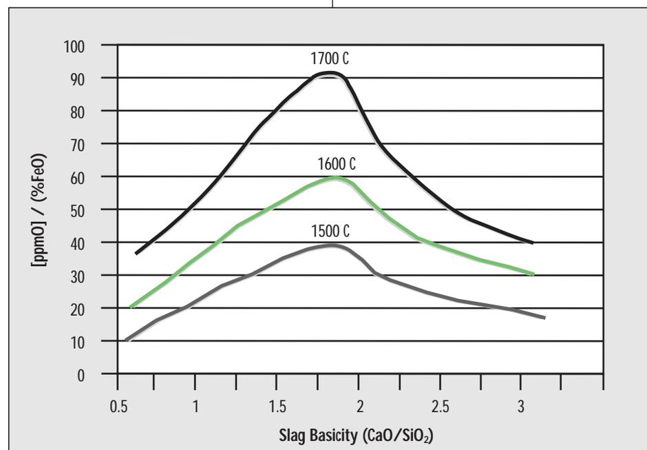
Figure 1 Equilibrium Ratio of FeO to Slag Basicity
