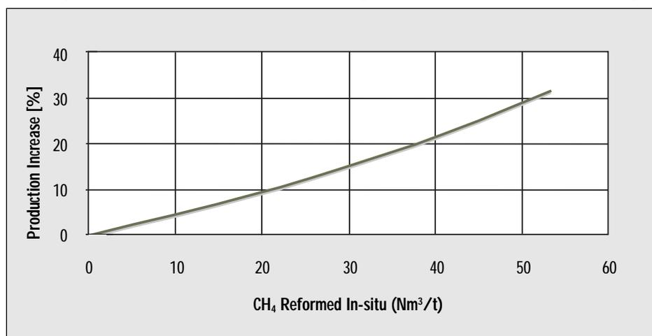
Figure 1 Production Increase with In-situ Reforming
