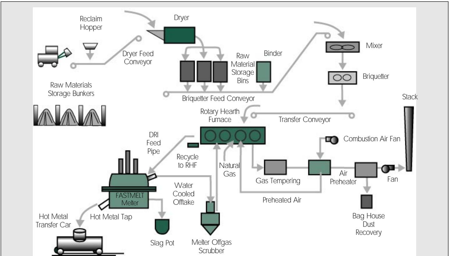
Figure 2 FASTMELT® process flowsheet
