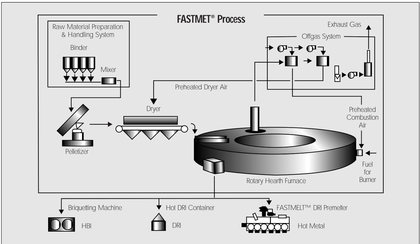
in place of natural gas. The raw material and the reductant are mixed, pelletized and dried, and then are transferred to a rotary hearth furnace (RHF) for direct reduction. The FASTMELT™ Process is the combination of the FASTMET Process and a specially designed DRI melter which melts continuously fed DRI and produces hot metal (FASTIRON™) with a controlled carbon content.
