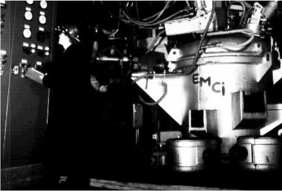
Figure 3 FASTMET Process Simulator and Melter
