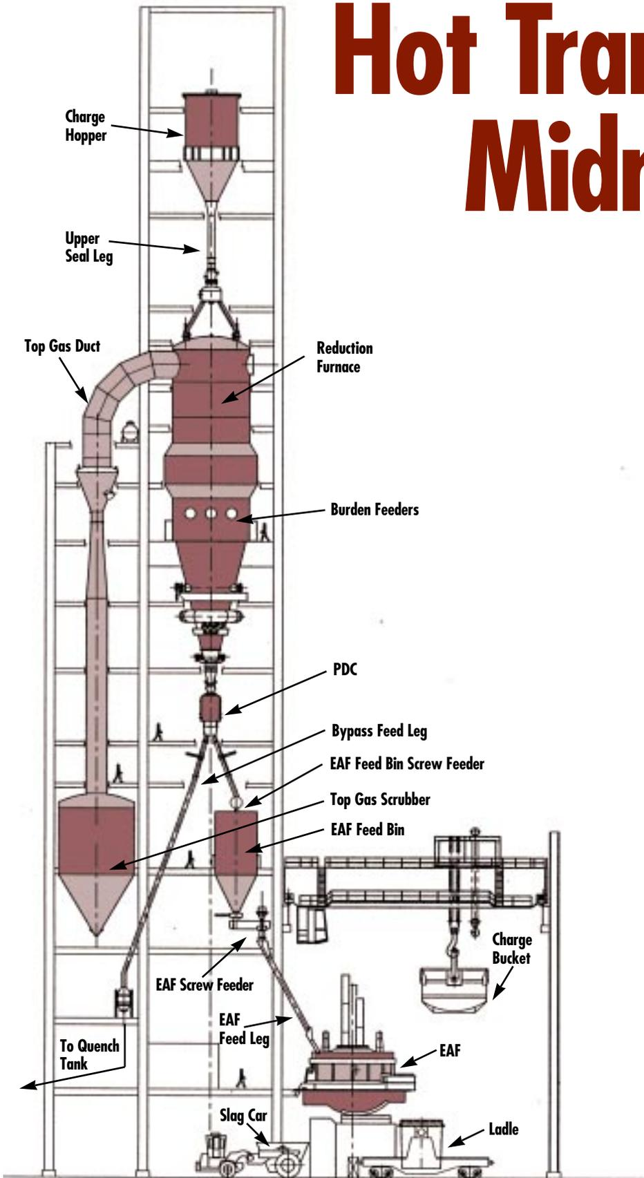
Figure 1 MIDREX Hot Charging System installed and connected to EAF Meltshop. This is an ideal situation because shorter travel time means less heat loss.
