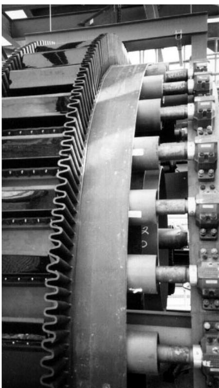
*The top of the vertical furnace feed conveyor*
